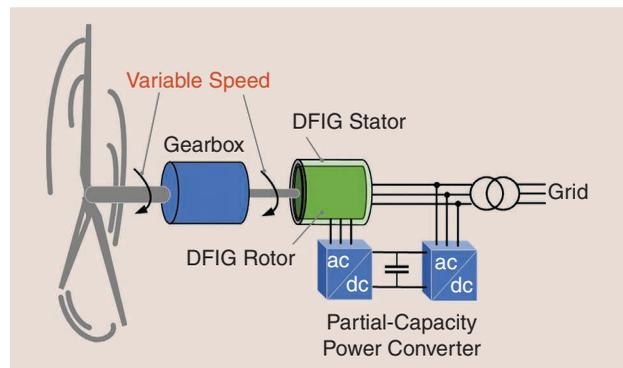
Figure 1. A Type-3 wind turbine topology.
